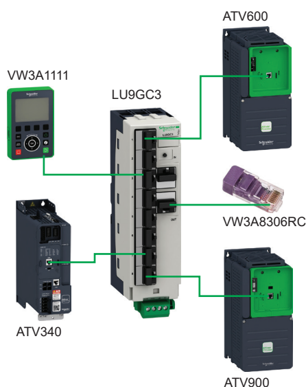
Example of multipoint screen architecture
